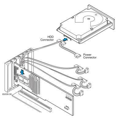
Figure 2.3 shows the SATA II device plug connector that connects a SAS RAID controller with internal connectors to the host receptable connector on a backplane. A SATA II connector consists of a signal connector and a power connector.
